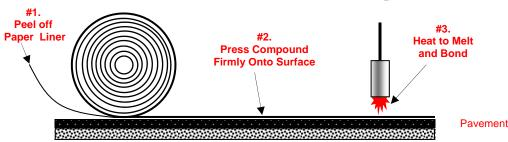
**DIRECTIONS:** Pavement must be clean, dry and free of dust prior to application of QuikJoint over-banding compound. Desired pavement temperature should be 40° F (4.4° C) and rising. Heat may be applied directly to pavement to dry and warm surface area to increase adhesion. For best results fill cracks wider than 1/16 inch with an approved crack filler level with pavement surface.
